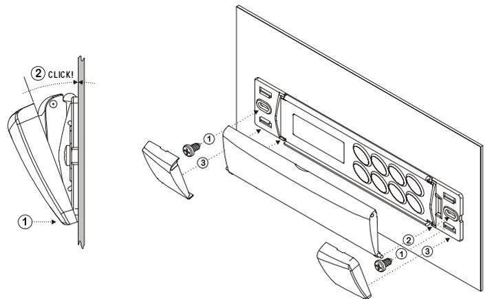
**MOUNTING WITH KEYBOARD COVER OPENING UPWARD**
